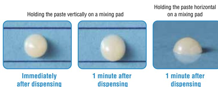
Fig.6: PASTE CONSISTENCY AFTER DISPENSING
